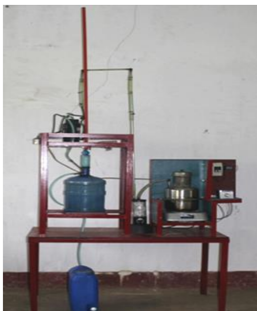
Figure 7: Set-up of the waste plastic oil converter
